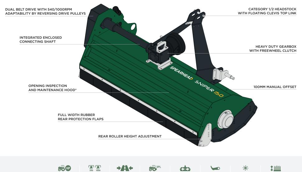
TRACTOR HP PTO SPEED TRANSPORT WIDTH **3 POINT LINKAGE** CUTTING WIDTH FLAIL TYPE NO. OF FLAILS CUTTING HEIGHT MOUNTING SNIPER 150 15hp (12kW) 540/1000rpm 1.67m (5' 6") 1.50m (4' 11") Heavy-duty 22 10mm - 50mm hammer flail (0.4" - 2")
